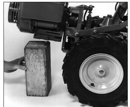
Figure 4-23: Block up engine.
